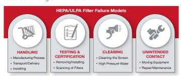
HEPA Filters typically fail due to some form of contact combined with the poor mechanical strength of the media.
