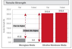
Results based on Test Standard DIN EN 29073-3.
