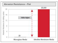
Results based on Test Standard DIN EN 12947-2.
