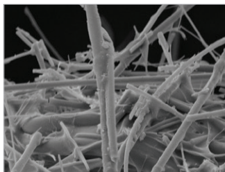
Fractured ultrafine microglass media fibers at fold tip @ 10,000x magnification.
