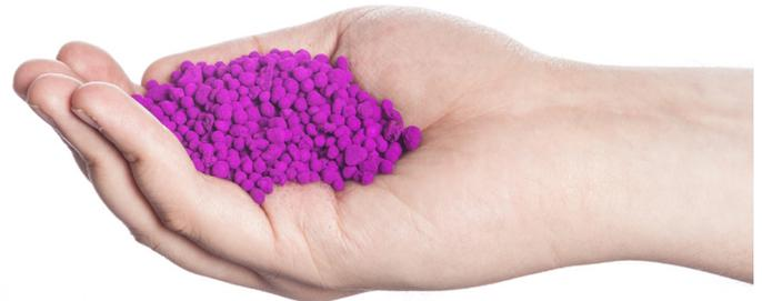
**Purafil Select Media (CHS)** consists of generally spherical, porous pellets formed from a combination of activated alumina and other binders, suitably impregnated with potassium permanganate (KMnO<sub>4</sub>). The potassium permanganate is applied during pellet formation such that it is uniformly distributed throughout the pellet volume and is completely available for reaction with target gases.
